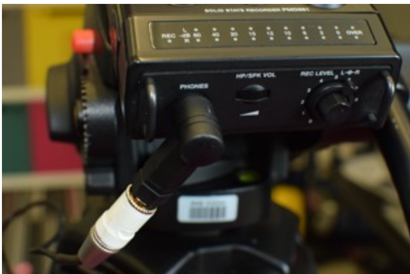
Plug Mix Pre D return cable into headphone socket of field recorder
