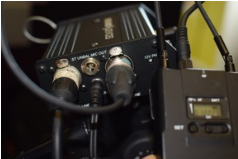
Radio mic receiver at freq A into channel 2 of Mix Pre D using OUTPUT not monitor jack .
