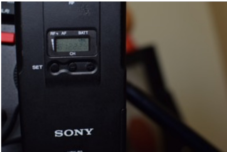
Radio mic receiver at freq A into channel 2 of Mix Pre D
